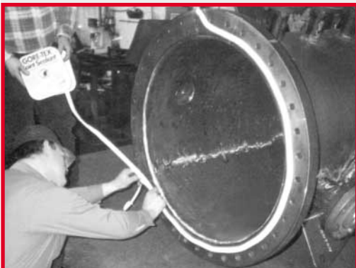
GORE-TEX® Joint Sealant is easy to install, even on vertical surfaces.
